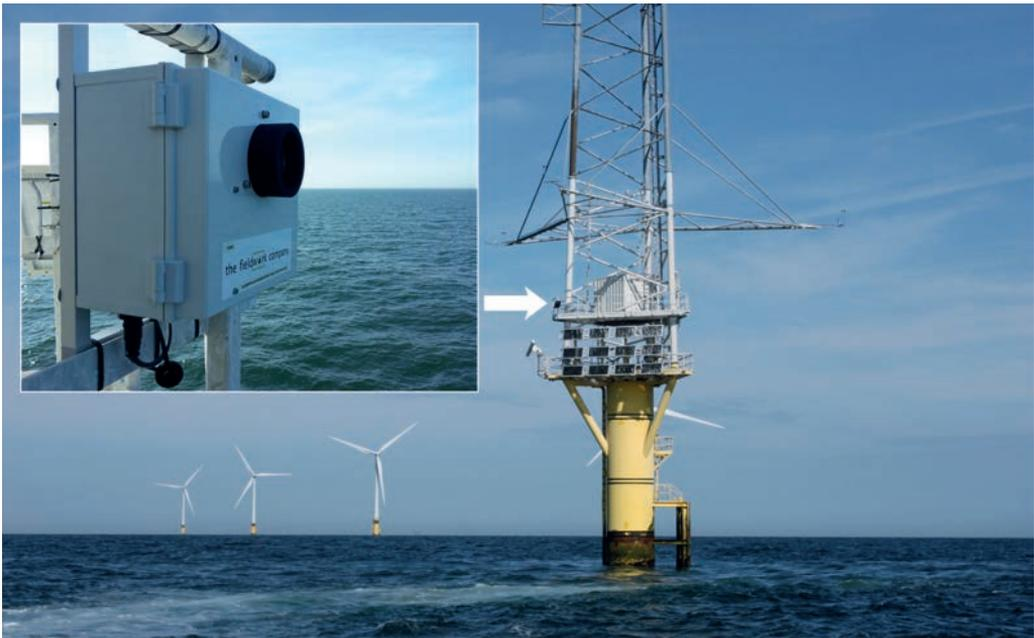
Figure 2. Ultrasonic recorder at the OWEZ meteorological mast. Photo: Hans Verdaat.
