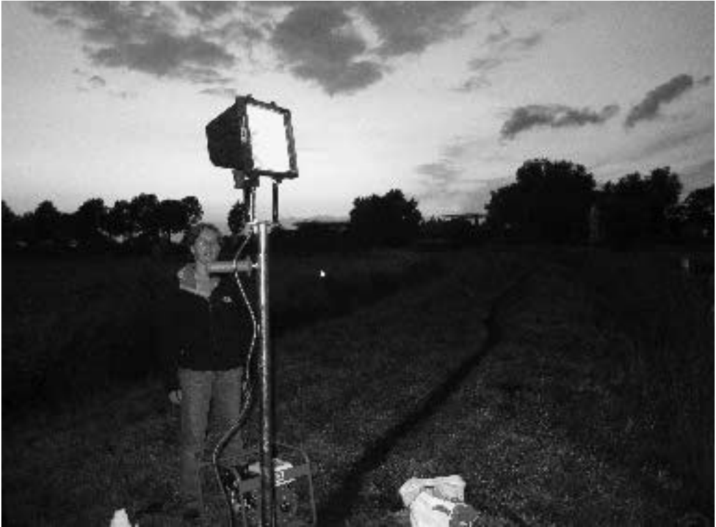
Photo 1. Experimental lighting consisted of a 1000 W halogen lamp, producing a beam of light between 1-30 Lux, with a diameter of approximately 10 m which was placed along the waterside of a commuting route of pond bats. Photograph: N. Goossens.
